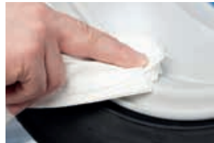
1. Cleaning and pre-treating the rim
