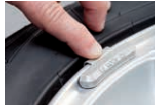
4. Checking the weight fitment
