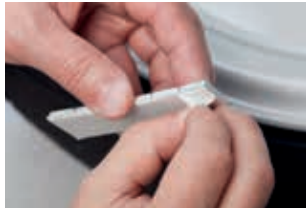
2. Select the correct adhesive weight size
