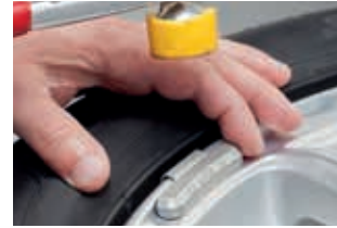
3. Installing the weight using a hammer
