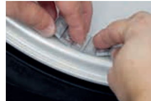
3. Applying the adhesive weight
