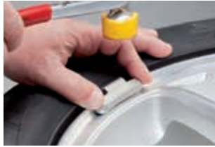
2. Placing the weight on the rim
