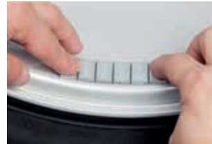
4. Securing the adhesive weight
