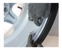
Adjust the adhesive weight to the rim radius with the protective film. The radius of the weight body and the rim must be at least in parallel to each other. It is even better if the radius of the weight body is less than that of the rim.
