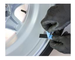
Remove the protective film from the adhesive tape after adjusting the weight to the rim radius. Do not touch the adhesive tape before attaching it to the wheel!
