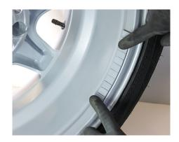
Now press the weight against the rim from the centre towards the outer edge. The pressure should be at least 100 kpa.
