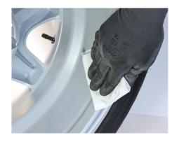
Ensure that the weight, rim and ambience temperatures are at last 16 °C. Clean the wheel rims with a suitable cleaning agent to avoid grease and silicone residue on the rim (e.g. isopropanol 70%).
