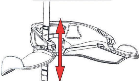
When feeding the pin into the desired slot, take extra care not to puncture the tether, and be sure the pin is aligned with the small hole in the back of the slot. Do not force the pin, it should easily screw in. Watch closely as you insert the pin into the loop to ensure that the pin fits inbetween the tethers, and not outside of them. When tightening the pin, do not overtighten as it will cause damage to the insert. **Tighten to 25 in. lbs.**
