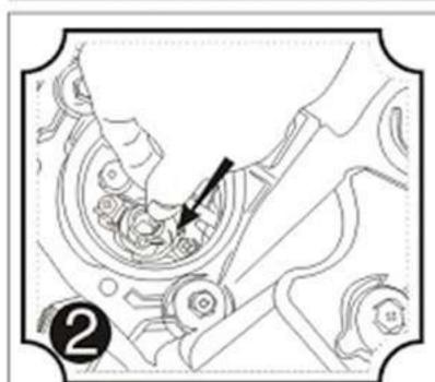
Align the collar of the bulb in the factory socket and use the metal clamp to lock it into place.
