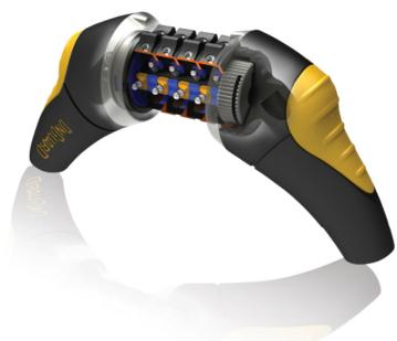
The Z-Cylinder offers high pick protection and features BumpBlock™ technology to render bump keys useless. Lock mechanism is encased in ultra-hardened steel to resist drilling or pulling.
