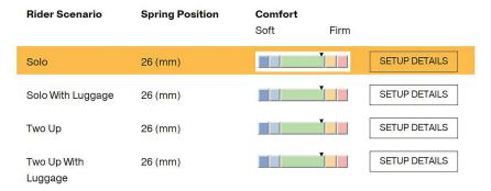
7. The "Spring Position" will tell you in millimeter the distance the preload collar should be from the bottom of the cylinder head for each scenario with your primary use highlighted in Gold.
