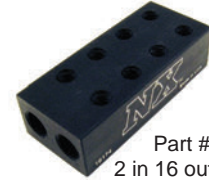
Part #16197 Black 1 in 4 out Compact Distributon Block (Shown with optional fittings) For AN outlet fittings use NX Part 16150 For compression outlet fittings use NX Part 16149
