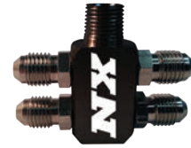
Part #16197 Black 1 in 4 out Compact Distributon Block (Shown with optional fittings) For AN outlet fittings use NX Part 16150 For compression outlet fittings use NX Part 16149
