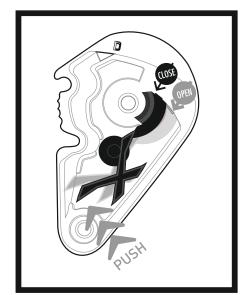
Block'N'Seal system with its automatically closure Spring button ensures smooth and waterproof seal every time you close the helmet Visor;
