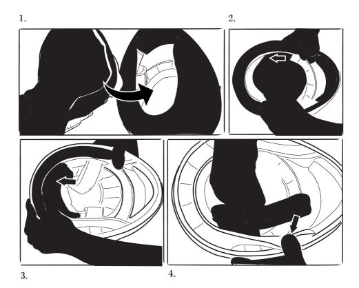
HOW TO REMOVE THE INNER LINING?
