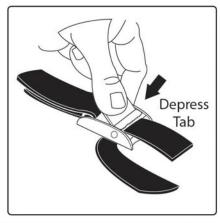
Pass the end of the strap through the cam buckle by pressing down on the aluminum tab and passing the strap through the back of the buckle and pulling tight.
