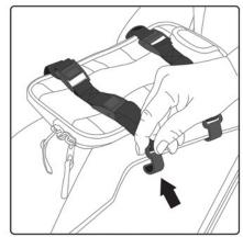
Place bag on front fender. Align so that the bag will not interfere with any moving part of the bike. Place the hooks around the edge of the fender. It might be necessary to remove some of the slack in the strap to move the hook closer to the fender.
