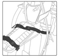
Once installed make sure that the bag is secure and free from any moving parts of the bike. Always be sure to check the bag before each ride and that all mounting points are still stable and correctly installed.
