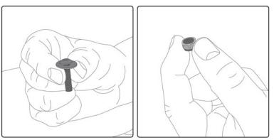
Using the provided hardware, place the washer around the bolt and pass through the bag and fender. Using a 4mm allen wrench for button head bolt and 10mm wench or socket for the nut, secure the bag to the fender. Tighten all bolts and make sure bag is stable before riding.
