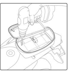
Once you bag is in place on your fender, using a 1/4" bit, drill 4 holes into the plastic bottom your bag and though the fender where you want your mounting points to be.
