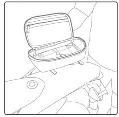
When lining up the bag on your rear fender, always be sure to check under the fender for any wires or cables so they do not get cut or damaged when drilling your mounting holes.
