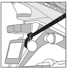
OPTIONAL STRAPS INCLUDED: If you do not have a plastic dual sport fender, use the 2 supplied straps with loops and wrap around a secure point on the vehicle and insert the strap thru the loop cinching tight. Then follow next step.
