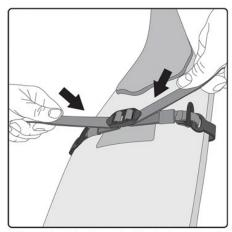
Secure both hooks under the fender and pull the straps tight as shown. Loop the straps thru the "D" ring near each hook.
