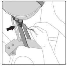
Loop front strap around frame or secure point thread thru buckle and pull until tight. Secure all loose end and keep away from moving or hot parts.
