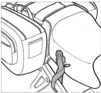
Using the strap with buckle on one side and loop on the opposite side, hook it or loop it around the frame, foot peg or secure body part and then back into the clip on the bag. You can also pass the buckle through the loop creating a noose to attach it around the frame or secure body part.
