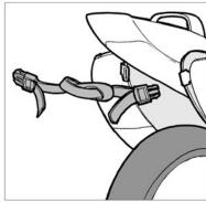
Depending on your bike's configuration, you may have to connect the two bags together with the side straps as shown. Position straps under the fender or licence plate bracket. Do not overtighten. Check the bags from the rear of bike to make sure they are not angled in or out. Bags should be as vertical as possible.
