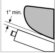
The saddlebags should be positioned with a minimum of 1" clearance above exhaust pipe (see diagram above). Although bottoms of bags have an aluminized heat shield, it will not protect from direct contact with your hot exhaust and is not covered by our warranty.
