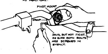
9. Remove telescope brackets now and loosely screw on locking nuts and replace telescope brackets on uprights.
