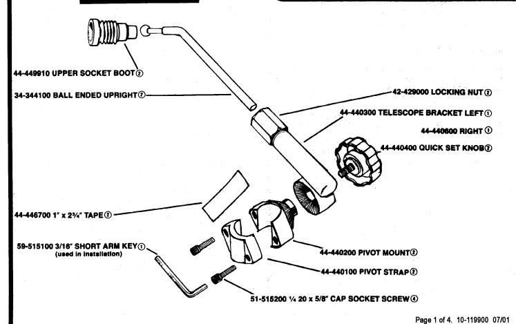
2. Use a padded surface or some other fixture to support the PLEXISTAR 2 or AIR-HAWK. Firmly grab the lower leg section and insert a lower "L" bracket with a twisting motion. Do both sides. If the fairing is colder than 65° -, it might be necessary to WARM the swivel and socket points with a hair dryer. DO NOT USE LUBRICANTS (EXCEPT) SALIVA OR WATER) ON ANY PART OF THE SCREEN OR HARDWARE!
