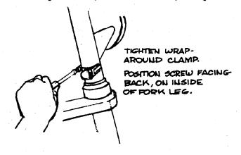
13. Place wrap-around clamp on knurled area of "L" bracket, push wing screw through and then insert and tighten into fork boss. TIGHTEN FORK CLAMPS AFTER wing screw is tight.
