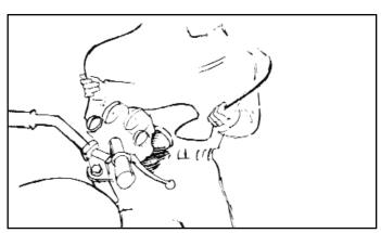
**5.** Select the left side Telescope Bracket and slide the Bracket onto the Upright. Repeat for right side.
