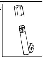
**10.** Reposition Plexifairing GT on motorcycle. Engage Telescope Bracket with Pivot Mount and secure with QuickSet Knob. HAND TIGHTEN LOCKING NUTS UNTIL FINAL ADJUSTMENT IS COMPLETE.
