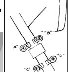
**12.** Thread Fork Clamp thru Fork Boss and tighten loosely around fork. Cosmetically it is preferable to have the screw of the Fork Clamp facing toward rider on inside of fork leg. Cut off excess strap with diagonal cutters after final adjustment.
