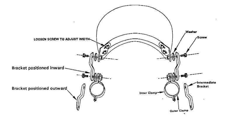
5. Assemble windshield hardware. Use the Fork Width measurement to determine position of the Adjustable Intermediate bracket to windshield.
