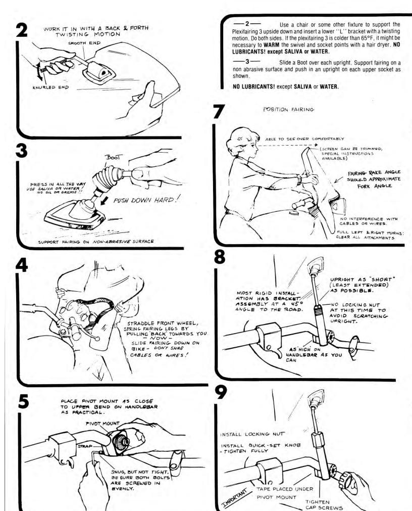
— 4 — Put motorcycle on center stand. Straddle front wheel and spring the Plexifairing 3 legs apart by pulling back on handlebar portions. Now slide fairing on bike. Be careful not to snag any control cables or loose wires. On some Hondas and Yamahas, bend the control cable loops out of the way. Legs should be behind turnsignals.
