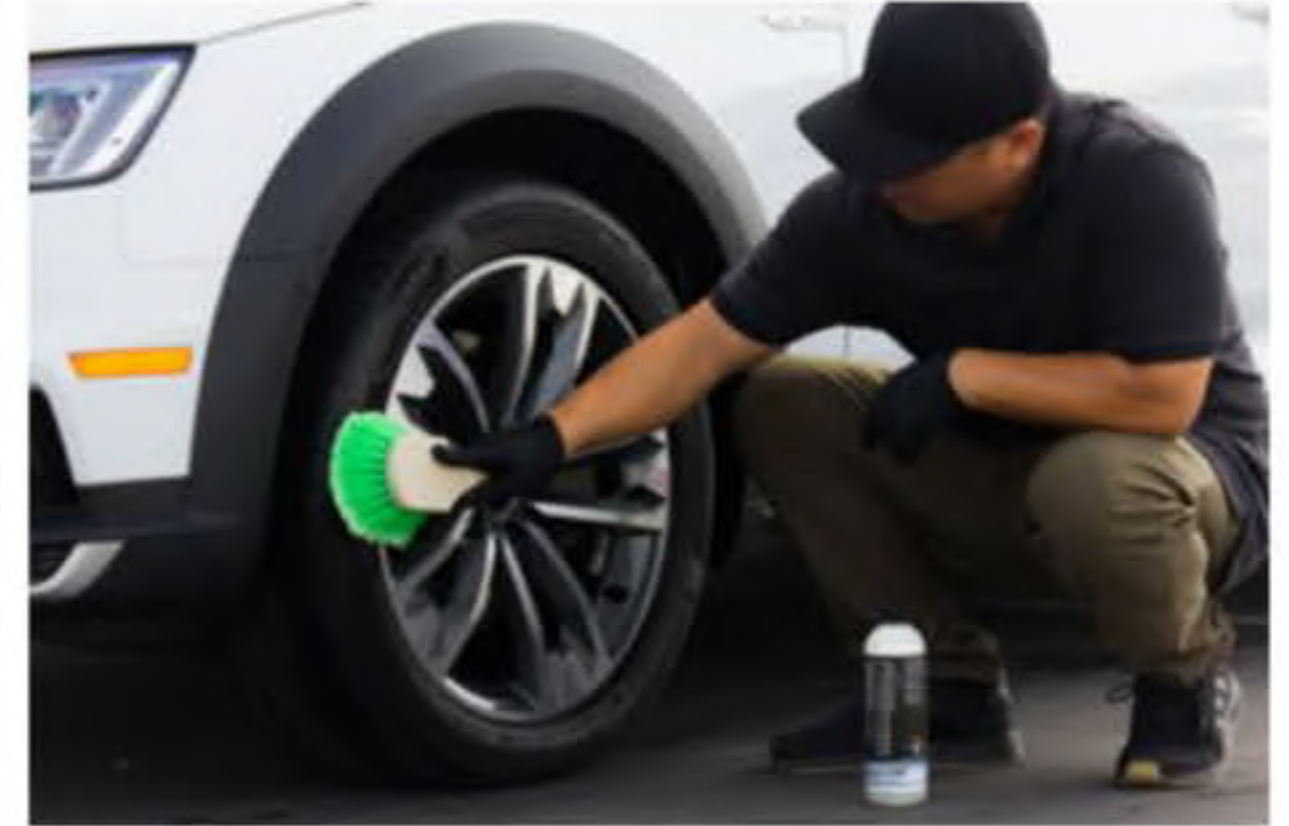
Step 3: Apply Multi Dress to wheel and spread evenly using wheel brush
