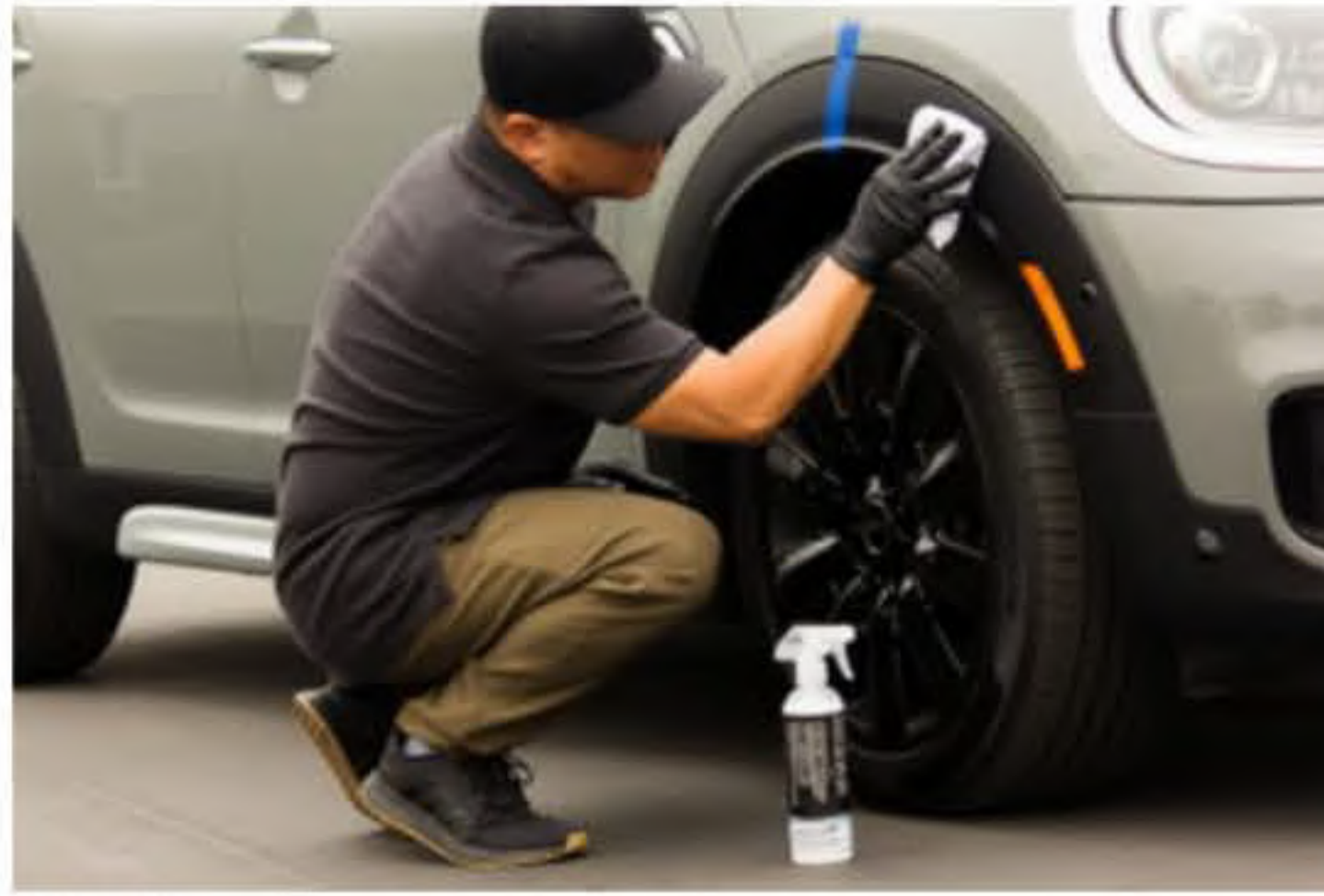
Step 2: Apply dressing to plastic surfaces using light to medium pressure. Reapply if necessary.
