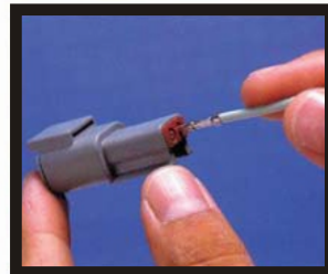
3. Hold the rear seal in place, as removing the contact will displace the seal.
