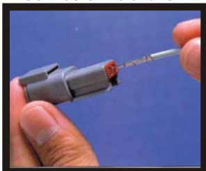
2. Hold the connector with the rear grommet facing you.
