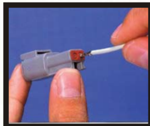
3. Push contact straight into the connector grommet until a "click" is felt. A slight tug will confirm that it is properly locked in place
