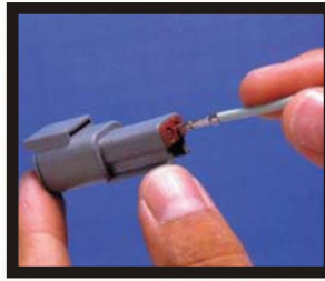
3. Hold the rear seal in place, as removing the contact will displace the seal.
