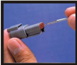
2. Hold the connector with the rear grommet facing you.
