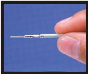
1. Grasp contact approximately 1" behind the contact barrel.
