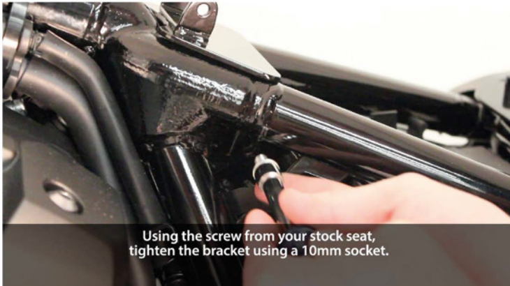
Now install the front seat hinge bracket by lining up the pins with the two holes in the front portion of the bike frame.
