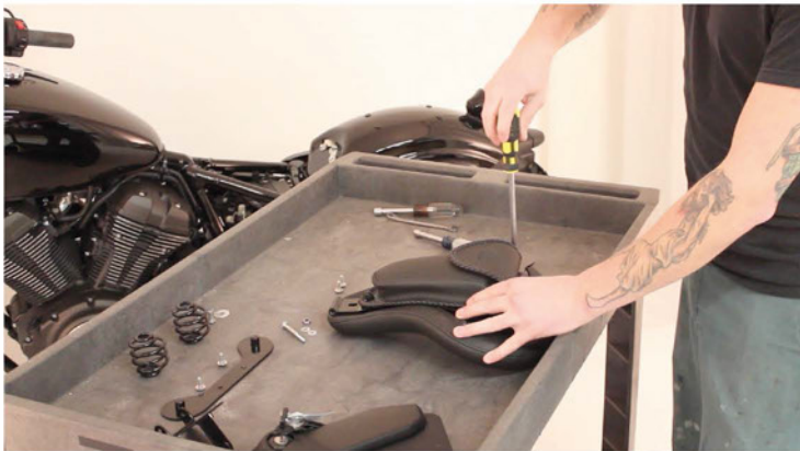
Using three 1/4"-20 x 5/8" screws, attach the plate to the seat starting with the two rear locations.
