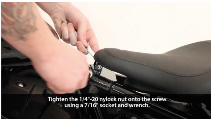
As you slide the 1/4"-28 x 2-1/4" hex cap screw through the bracket, position a white nylon washer on each side of the nose of the seat mounting plate.
