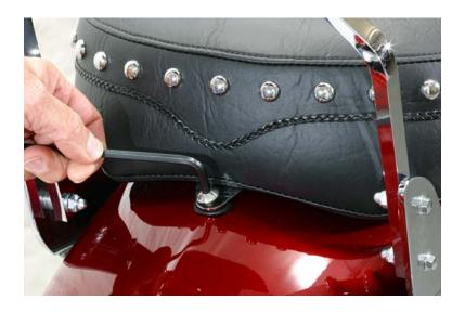
4. Push the passenger seat forward until the rear bracket aligns with the fender mount. Secure the bracket to the fender with the stock 6mm rear screw.
