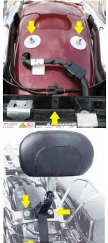
mounts, and the forward mount to the hole with the threaded clip. Secure the base with the two stock bolts or nuts (fender) and the supplied 1/4"-20 x 3/4" bolt and washer (frame).
