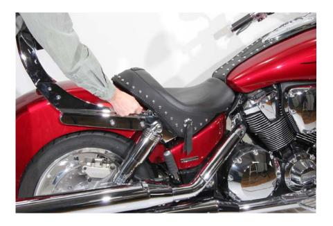
3. Slide the passenger's front bracket into the receiver on the back of the solo.
