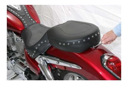
6. Place the remaining nylon washer under the passenger seat's rear bracket and secure with the stock acorn nut. Tighten securely.
