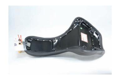
3. Engage nose tab at front of seat, then align and secure the rear mounting tab to the fender.
