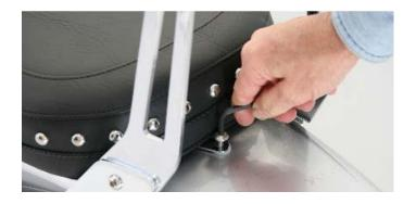
6. Place the white nylon washer under the passenger seat's rear bracket and secure with the stock 6mm bolt. Tighten securely using a 5mm Allen wrench.
