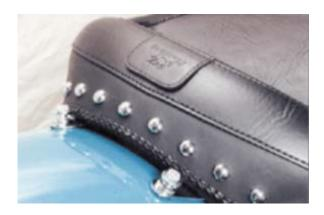
4. Align the passenger seat so that the two slotted brackets engage the spool washers. Push the passenger seat fully forward.
