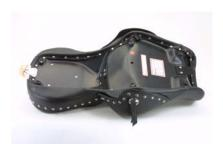
3. Slide the seat back and up to remove from the motorcycle.
