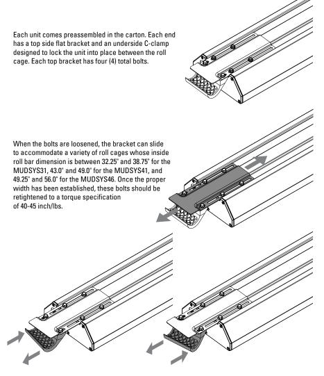
Each C-bracket has two (2) total bolts. These bolts can be loosened to adjust the clamp angle allowing it to mount to a variety of roll cages including those that are angled.
