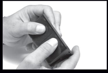
Step 10) Place reeds on outside surface and press on to locating tabs.
