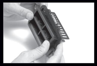
Step 11) With reeds in place, push reed cage through flange until locating tabs snap into their openings.
