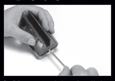
Step 3) To remove center reeds, place small screwdriver into slot above retainer bar at a 45 degree angle.
