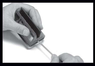
Step 9) Using a screwdriver or similar tool, push retainer bar flush with reed cage surface.
