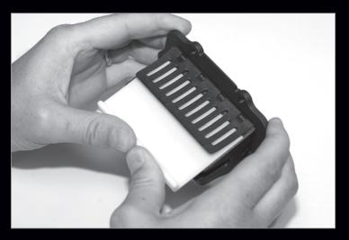
Step 1a) For reed valves with extended reed stops, insert tool between reed and reed stop and push cage firmly.
