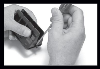
Step 4) Using light pressure pry retaining bar out gradually until retaining bar can be easily removed by hand.
