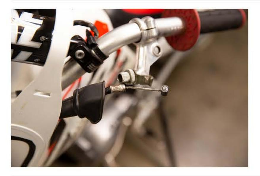
You service manual will also have detailed specifications about cable adjustment and in some cases, proper cable slack, which is also critical to the proper and safe function of your motorcycle.
