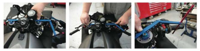
Turn the tool over, and place it back into the same position on the forks, but this time the alignment notch will be on the opposite fork. Pay attention to the indicating rod, and do not allow the angle of the second- ary arm to change. If you are not able to place the tool properly without the indicating rod contacting the handlebar, that means the handlebar is positioned too far back.
