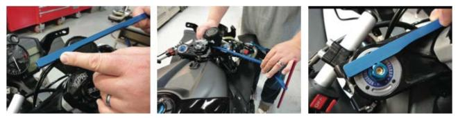
Next, align the notch on the end of the main arm with the center of the fork tube that is opposite from the handlebar you are measuring. Once the main arm is in this location, do not allow it to move through the next step.
