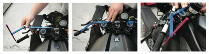
If you place the tool, and there is a space between the indicating rod and the handlebar, that means the handlebar is too far forward. Make adjustments to that handlebar, and check again with the tool. Move the tool to each side several times, and make adjustments as necessary to the sweep of the handlebars.
