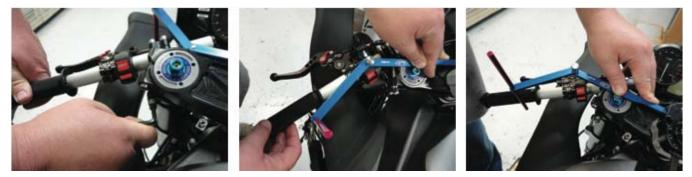
When the indicating rod lightly contacts both sides evenly, your handlebars are adjusted properly with identical sweep on both sides.
