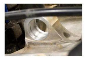
5. Carefully clean the inside of the swing arm bearing surface using fine scotch-brite and contact cleaner to remove any burrs or corrosion.
