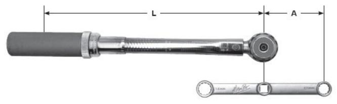
NOTE: When using 3 inches for distance "A", torque wrench and torque adapter must be in line. If the adapter is positioned at an angle to the torque wrench, distance "A" will be decreased. When the adapter is at a 90-degree angle to the torque wrench, distance "A" will be equal to zero (0).
