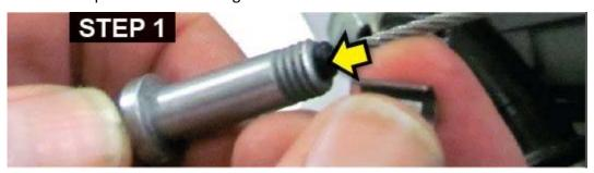
• Gently pry open the adapter just enough to install onto clutch cable elbow fi tting at engine.
