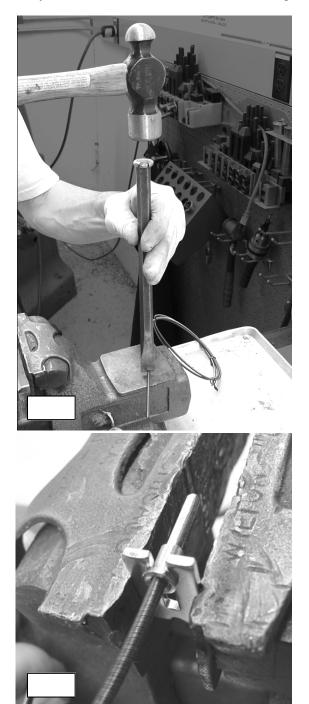
2. Deduct 5/8" (16mm) from measurement and cut new cable to this length. Be sure to cut round end of cable - do not cut squared end. Best way to cut the new inner cable is to use a sharp chisel and hammer. Use a flat metal surface and place the chisel on the cable. Strike the chisel with hammer using a strong blow. USE EYE PROTECTION. (See figure 1)
