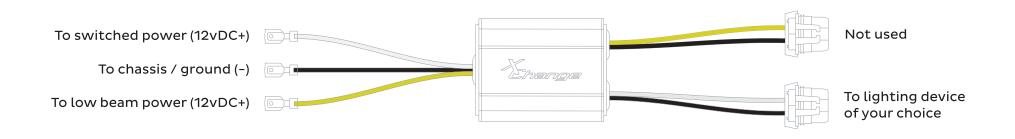
THIS WIRING SCHEMATIC IS USED FOR THE INSTALLATIONS WHERE THE RUNNING LIGHT IS ILLUMINATED CONSTANTLY BASED ON A POWER SOURCE'S SIGNAL. WHEN THE VEHICLE'S INDICATOR IS SWITCHED ON, THE ILLUMINATED LIGHTING DEVICE TURNS OFF, AND A SECOND LIGHTING DEVICE IS ILLUMINATED CONCURRENT WITH THE INDICATOR'S TIMED SEQUENCE. ONCE TURNED OFF, THE ORIGINAL RUNNING LIGHT RETURNS AFTER A BRIEF PAUSE.
