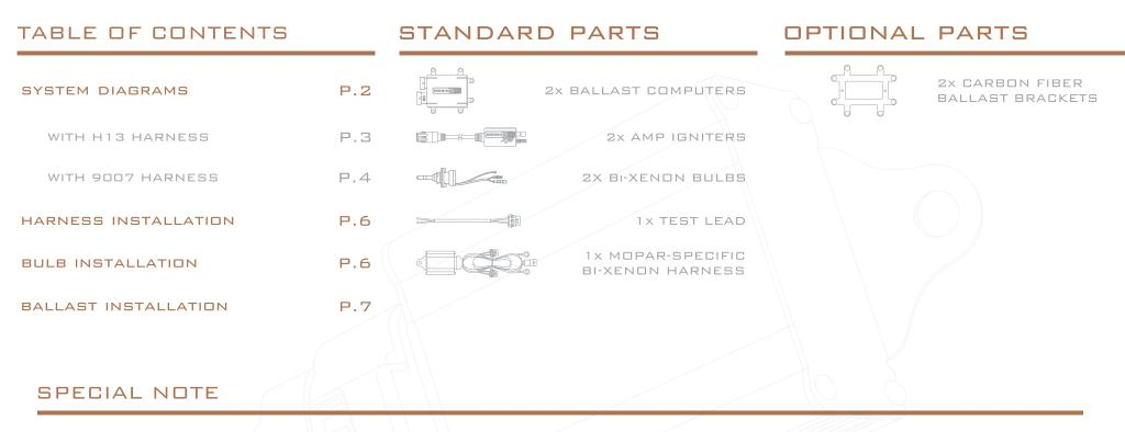
The Mopar-Specific harness is designed specifically to eliminate your vehicle's "bulb out" error. Due to the complexity of your vehicle's CANBUS bulb monitoring system, this is the most compatible harness available. If you have any persistent issues related to this system after installation, consult your Authorized Morimoto dealer for further support.
