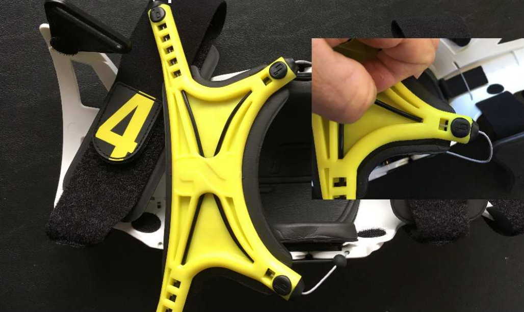
Step 37 - Push cable housing through lower leg, and pull cable and housing back through tendon back plate as shown
