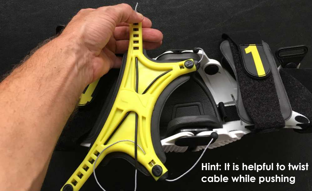
Step 37 - Push cable housing through lower leg, and pull cable and housing back through tendon back plate as shown
