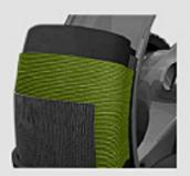
Stiff ply material and Metzeler 0° steel belt technology for high lateral stiffness
