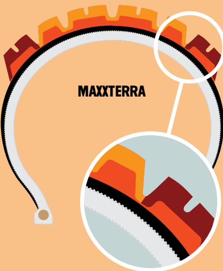
An intermediate compound configuration used in select mountain tires. 3C MaxxTerra is softer and offers more traction than 3C MaxxSpeed, yet provides better treadwear and less rolling resistance than MaxxGrip.
