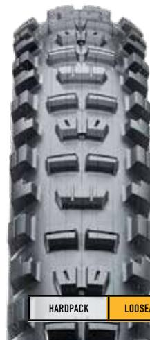
The Minion DHR II is the perfect counterpart to the DHF, and it's now available for the most capable plus bikes on the market. Ramped center knobs decrease rolling resistance compared to the DHF while improving braking traction.
