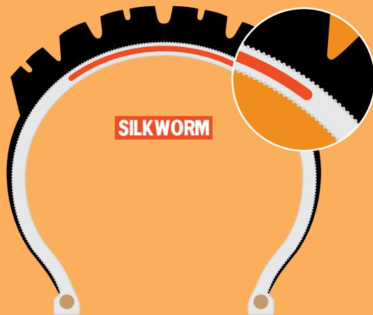
SilkWorm is an exclusive material incorporated into the casing of select models, increasing puncture and tear resistance. SilkWorm is featured under the tread as a breaker.
