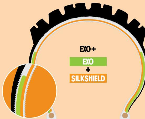
EXO+ combines two of our best puncture protection materials: SilkShield and EXO. The SilkShield layer runs from bead-to-bead with a layer of EXO along the sidewalls. Together, they create EXO+, improving tread puncture protection by 27%; sidewall durability by 51%; and resistance to pinch flats by 28%.
