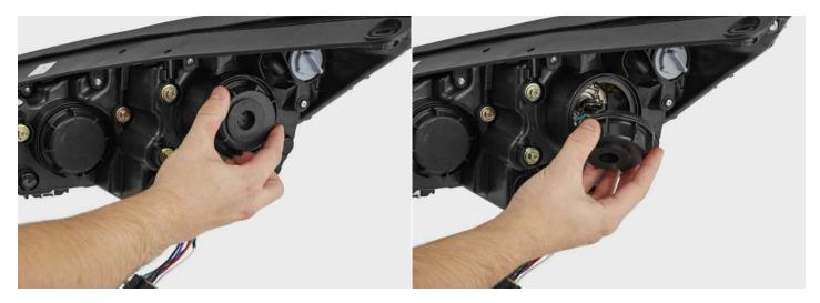
© Remove the bulb from the headlight assembly.
