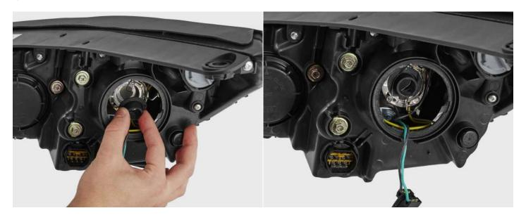
$\ensuremath{\mathbb{R}}$  Insert the bulb into the secured collar and lock the bulb with a twist.
