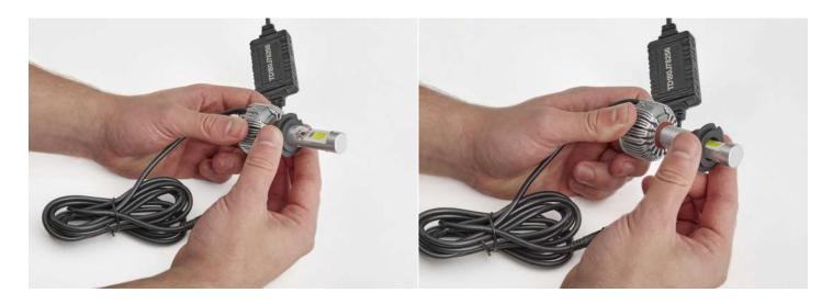
Place the collar into the bulb socket and secure it.
