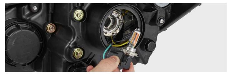
© Disconnect all wiring from the bulb base.
