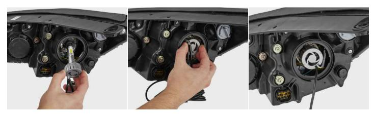
© Do not re install OEM dust covers, to allow for adequate cooling of conversion bulbs
