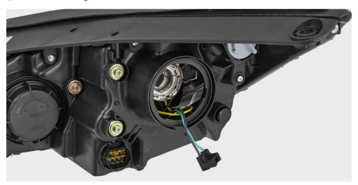
(H) Connect all the components for the driver and passenger side bulbs.
