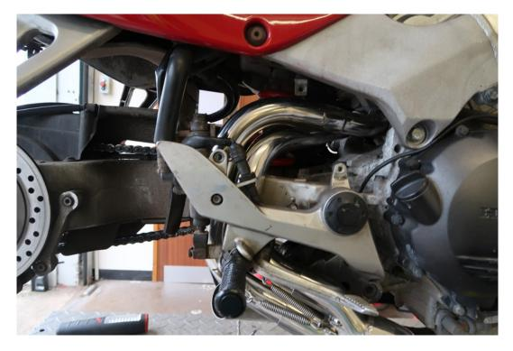
Insert the exhaust gaskets (supplied) into the front exhaust ports, use a small amount of exhaust paste to hold them into the ports if required.
