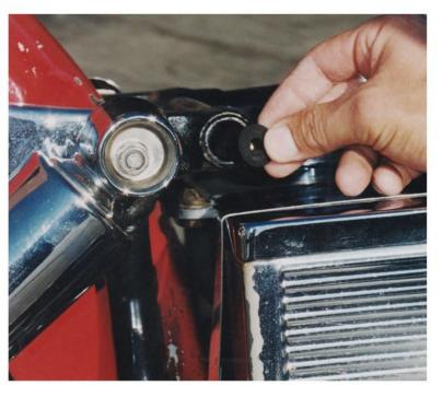
**B.** We've made bolting your new seat to the frame effortless. Simply insert the two rubber "plugs" into the two holes in your frame.
