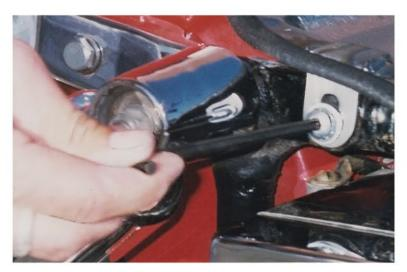
**C.** Slide the seat down over the plugs. Line up the brackets with the bolts and washers provided and tighten the bolts. When the seat is secure, stop tightening. **DO NOT OVER TIGHTEN.**
