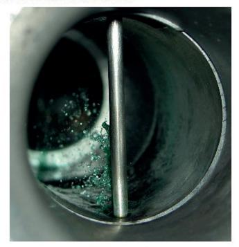
**The Best Throttle Response:** The smooth, tapered bore design creates the fastest air speeds of any carburetor. Unlike a choked down keyhole design, our products are designed to flow the most air at the highest velocity. Lectrons are also the only carburetor with the fuel pickup tube always under vacuum (on the engine side of the slide). That means it is always full of fuel and adjusting float height for throttle response is a thing of the past.
