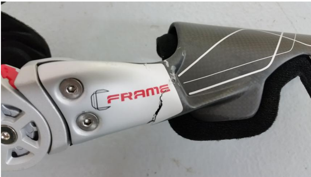
Figure 4-10: Fracture of carbon shin load pad strut at force above minimum required force of 682 N and below maximum allowable force of 3780 N
