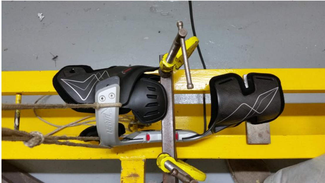
Figure 4-7: Hyperextension and Femoral Tolerance Test Setup Top View
