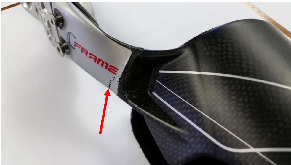
Figure 4-8: Fracture of carbon shin load pad strut at force above minimum required force of 416.5 N and below maximum allowable force of 750 N
