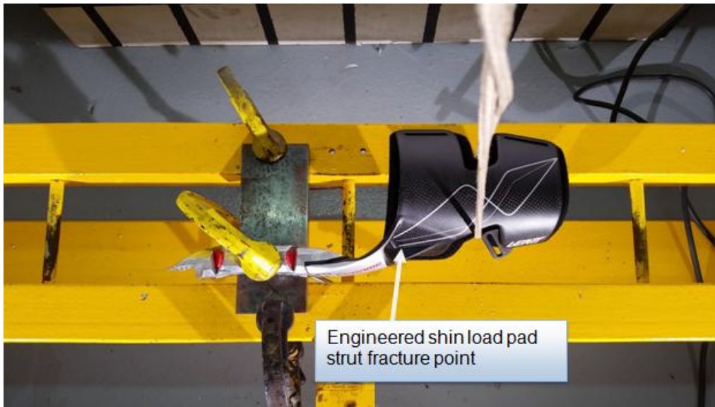
Figure 4-5: Hyperextension and Tibial Tolerance Test Setup Top View
