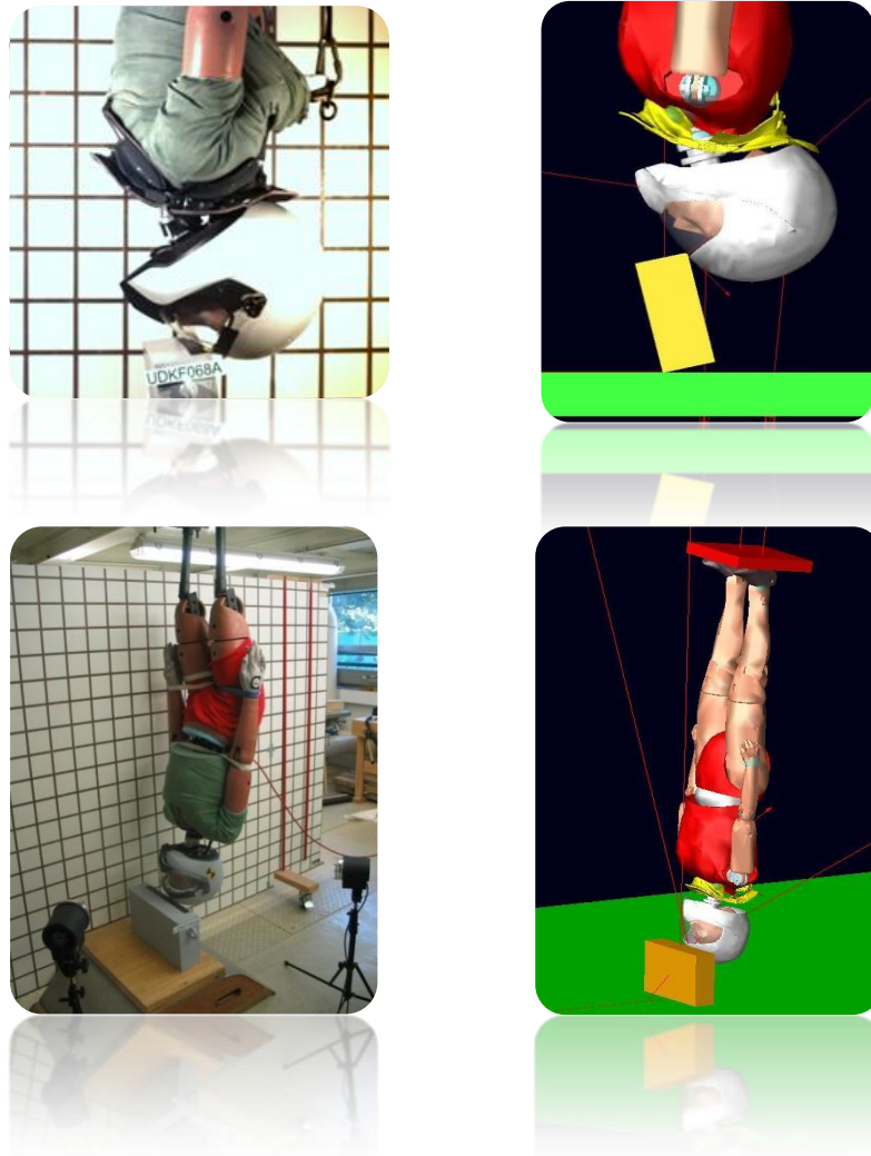
Figure 4-2: Pendulum test and simulation setup
