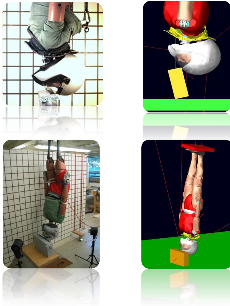
Figure 4-2: Pendulum test and simulation setup
